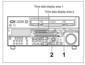
**1** Press the RECORDER button or PLAYER button to select the VTR on which you wish to check the edit point.
